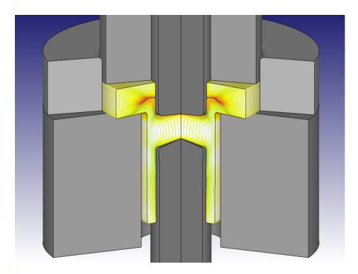
A fastener lap is clearly shown during the final operation of a cold formed automotive part. The actual part exhibited a lap that accurately matched the simulation results. Results such as strain (shown), stress, damage and temperature can be evaluated throughout the forming process. The FLOWNET tool (green lines) allows for the prediction of grain flow within a part.
