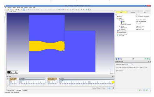
The DEFORM Multiple Operation environment allows for the automatic simulation of  $entire\ process\ sequences. \quad These\ are\ defined\ using\ a\ mix\ of\ flowchart,\ wizard-based$ and advanced menus. The hot forging process shown above was simulated, from start to finish, with a single click of the 'Run' button.
