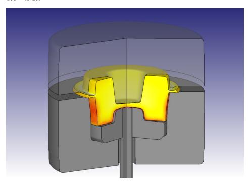
FORMING EXPRESS (2D) is frequently used to simulate manufacturing operations like the hot forging process shown above. Results include deformed shape, die fill, defects, part/die temperatures, strain, forming load and more. Die stress analysis facilitates troubleshooting of die failures and optimization of tool life.
